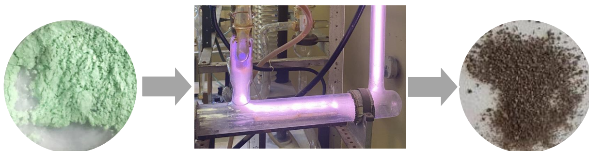
Fig.1. Cu-supported Al-Zr catalyst before and after glow discharge Ar-plasma.
